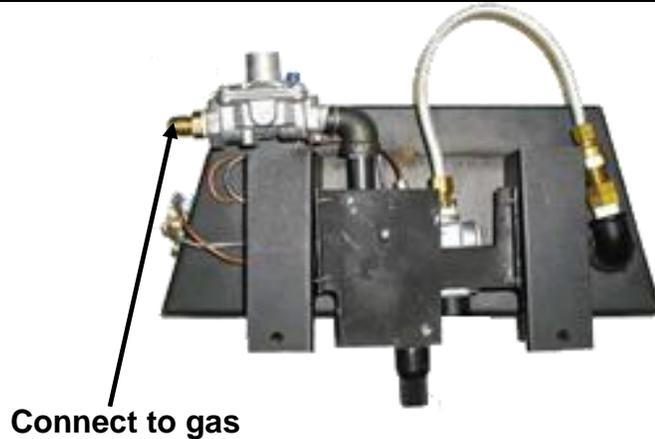
**IMPORTANT:** The minimum inlet supply pressure for the purpose of input adjustment is 5.0 inches (natural gas) 11 inches (propane gas) in water column. The maximum inlet supply pressure is 10.5 inches (natural gas) 13 inches (propane gas) in water column.
